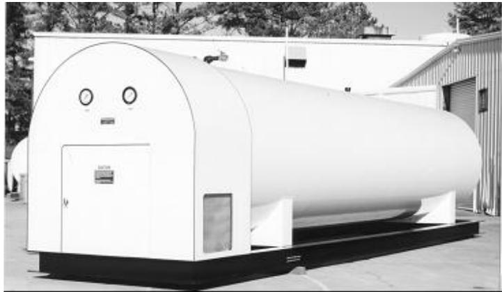
Figure 11—Bulk liquid carbon dioxide container
