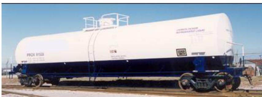
**Figure 7—Liquid carbon dioxide tank car**
