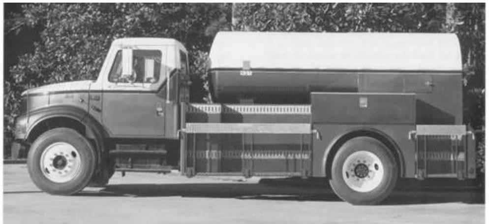
Figure 9—Liquid carbon dioxide cargo tank (straight truck)
