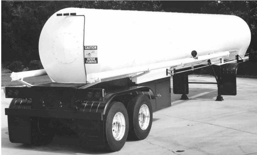
Figure 8—Liquid carbon dioxide cargo tank
